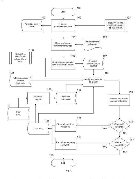
Fig.1. Illustration of the overall process flow of the invention
